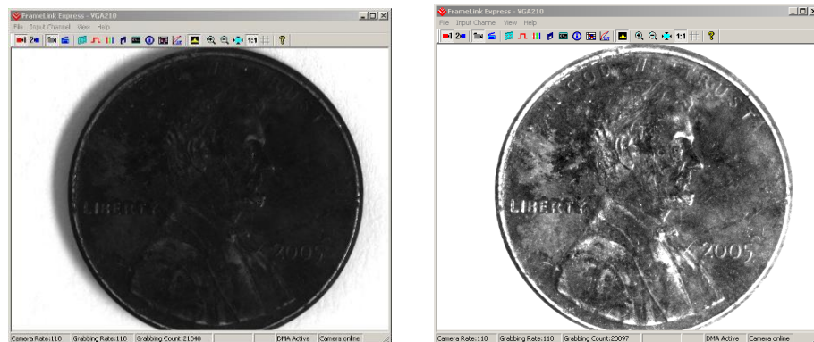
Figure 3.3 – Original and processed image with threshold and gray scale stretch.
