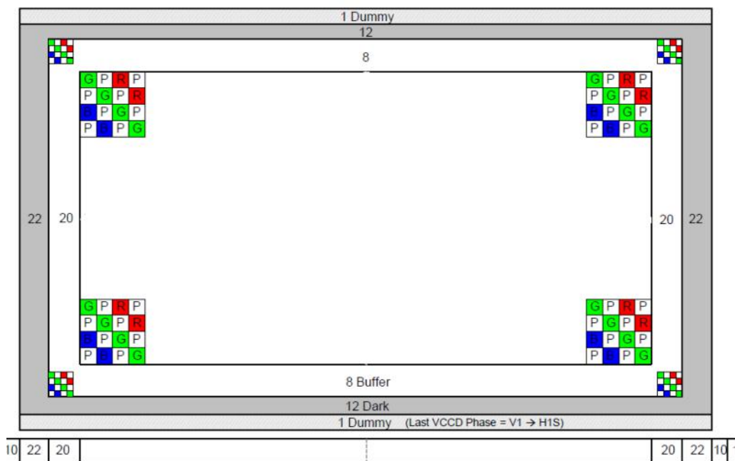
Figure 1.0b – Kodak TRUESENSE color filter interline CCD pixel structure.
