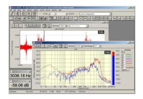
Cursor Measurements: Absolute, Differential (Ctrl key), Harmonic cursors (Shift key), Sideband cursors (Ctrl + Shift key)
