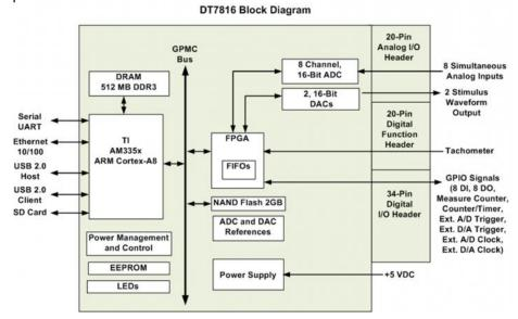
Figure 2. The DT7816 block diagram shows the board with the TI AM335x ARM Cortex-A8 processor, FPGA, memory and support peripherals as well as interfaces for a USB host and client, Ethernet, power, SD card, A/D, D/A, digital I/O, tachometer, and counters.
