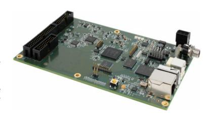
Figure 1. The DT7816 provides 8 analog inputs, 2 analog outputs, DIO, C/T, tachometer, and measure counter functions along with an embedded ARM processor for real-time processing and analysis of DAQ measurements.
