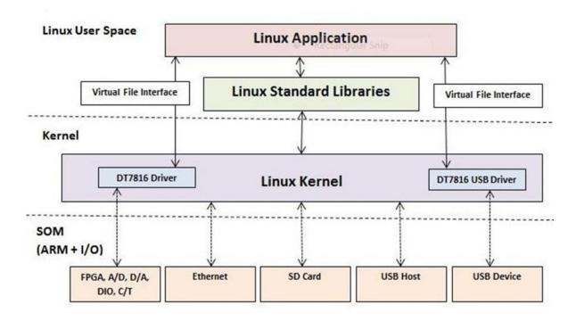
Figure 4. The DT7816 runs Linux 3.12 with custom loadable kernel modules, i.e., "device drivers" for the board hardware. These "drivers" expose the functionality of the board to Linux user space applications.
