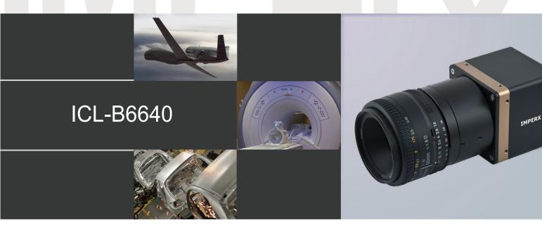
IMPERX ICL-B6640 is an advanced progressive scan, fully programmable CCD camera designed for imaging applications that require high speed, brilliant images, powerful features and flexibility. The camera is small, light weight, and built around the TRUESENSE Imaging KAI-29050, 4-tap, 5.5 micron interline transfer CCD image sensor with a 43.47mm optical format.
