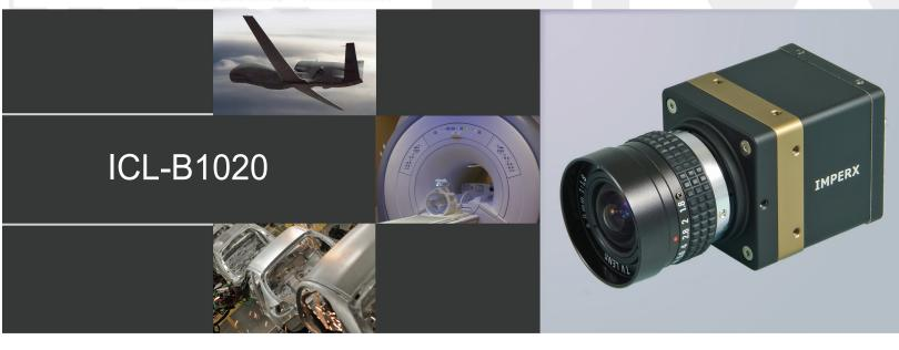
The ICL-B1020 is an advanced progressive scan, fully programmable CCD camera designed for imaging applications that require high quality images, powerful features and flexibility. The camera is small, light weight, and built around Kodak's KAI-01050 5.5 micron Interline Transfer CCD image sensor with a 1/2" optical format.
