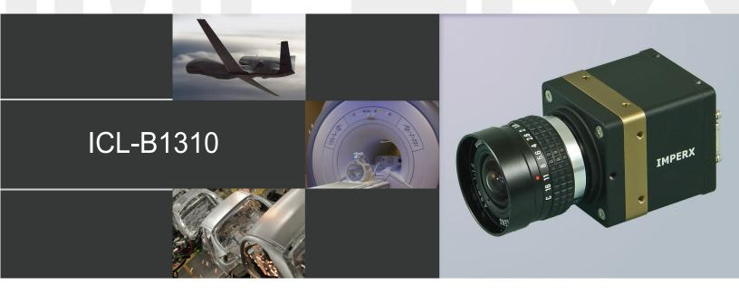
The ICL-B1310 is an advanced progressive scan, fully programmable CCD camera designed for imaging applications that require high quality images, powerful features and flexibility. The camera is small, light weight, and built around SONY's ICX 445 3.75 micron Interline Transfer CCD image sensor with a 1/3" optical format.
