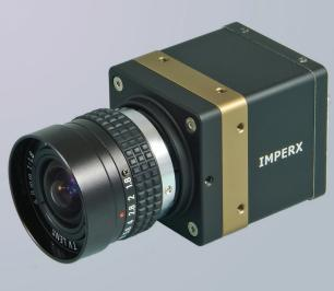
The ICL-B1320 is an advanced progressive scan, fully programmable CCD camera designed for imaging applications that require high quality images, powerful features and flexibility. The camera is small, light weight, and built around Kodak's KAI-01150 5.5 micron Interline Transfer CCD image sensor with a 1/2" optical format.
