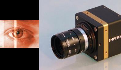
The **ICL-B0610** is an advanced high-speed progressive scan, fully programmable CCD camera designed for imaging applications that require high frame rates, high quality images, and powerful features and flexibility. The camera has a small size, light weight, and is built around Kodak's KAI-0340S Interline transfer CCD image sensor with a 1/3" optical format. ICL-B0610 is available with CameraLink output (PoCL compliant).
