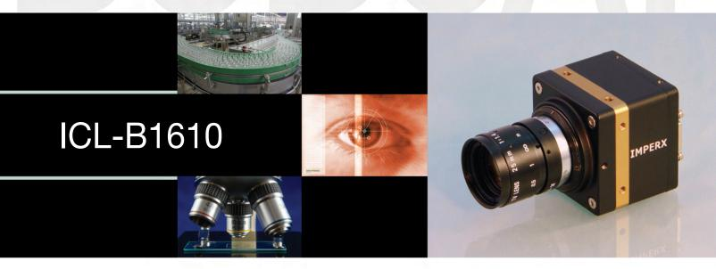
The **ICL-B1610** is an advanced high-speed progressive scan, fully programmable CCD camera designed for imaging applications that require high frame rates, high quality images, and powerful features and flexibility. The camera has a small size, light weight, and is built around SONY'S ICX-274 Interline transfer CCD image sensor with a 1/1.8" optical format. ICL-B1610 is available with CameraLink output (PoCL support).
