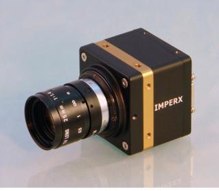
The **ICL-B1620** is an advanced high-speed progressive scan, fully programmable CCD camera designed for imaging applications that require high frame rates, high quality images, and powerful features and flexibility. The camera has a small size, light weight, and is built around Kodak's KAI-2020 Interline transfer CCD image sensor with a 1.0" optical format. ICL-B1620 is available with CameraLink output (PoCL compliant).
