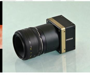
The **ICL-B2020** is an advanced high-speed progressive scan, fully programmable CCD camera designed for imaging applications that require high frame rates, high quality images, and powerful features and flexibility. The camera has a small size, light weight, and is built around Kodak's KAI-4022 Interline transfer CCD image sensor with a 1.3" optical format (21.5 mm image diagonal). ICL-B2020 is available with CameraLink output.
