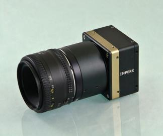
The **ICL-B4020** is an advanced high-speed progressive scan, fully programmable CCD camera designed for imaging applications that require high frame rates, high quality images, and powerful features and flexibility. The camera has a small size, light weight, and is built around Kodak's KAI-11002 Interline transfer CCD image sensor with a 43.3 mm image diagonal. ICL-B4020 is available with CameraLink output.
