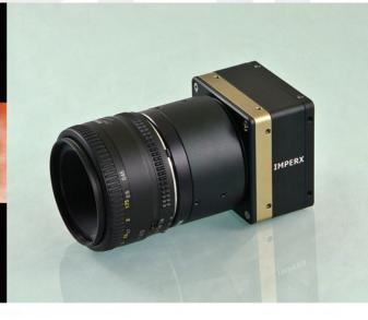
The **ICL-B4820** is an advanced high-speed progressive scan, fully programmable CCD camera designed for imaging applications that require high frame rates, high quality images, and powerful features and flexibility. The camera has a small size, light weight, and is built around Kodak's KAI-16000 Interline transfer CCD image sensor with a 43.3 mm image diagonal. ICL-B4820 is available with CameraLink output.
