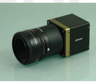
The **IGV-B4820** is an advanced high-speed progressive scan, fully programmable CCD camera designed for imaging applications that require high frame rates, high quality images, and powerful features and flexibility. The camera has a small size, light weight, and is built around Kodak's KAI-16000 Interline transfer CCD image sensor with a 43.3 mm image diagonal. IGV-B4820 is available with Ethernet output (GigEVision compliant).
