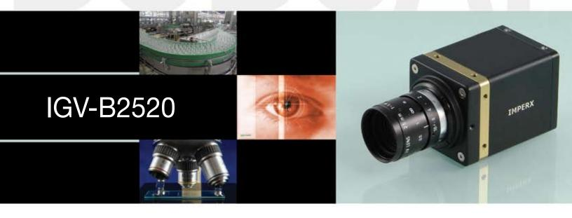
The **IGV-B2520** is an advanced high-speed progressive scan, fully programmable CCD camera designed for imaging applications that require high frame rates, high quality images, and powerful features and flexibility. The camera has a small size, light weight, and is built around SONY'S ICX-625 Interline transfer CCD image sensor with a 2/3" optical format. IGV-B2520 is available with Ethernet output (GigEVision compliant).
