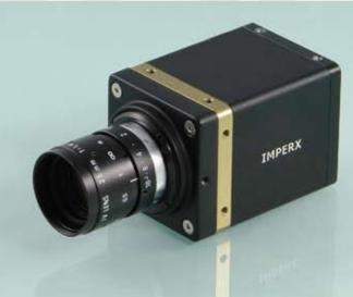
The **IGV-B1410** is an advanced high-speed progressive scan, fully programmable CCD camera designed for imaging applications that require high frame rates, high quality images, and powerful features and flexibility. The camera has a small size, light weight, and is built around SONY'S ICX-285 Interline transfer CCD image sensor with a 2/3" optical format. IGV-B1410 is available with Ethernet output (GigEVision compliant).
