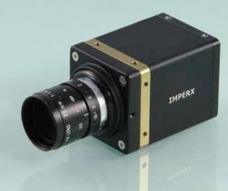
The **IGV-B0620** is an advanced high-speed progressive scan, fully programmable CCD camera designed for imaging applications that require high frame rates, high quality images, and powerful features and flexibility. The camera has a small size, light weight, and is built around Kodak's KAI-0340D Interline transfer CCD image sensor with a 1/3" optical format. IGV-B0620 is available with Ethernet output (GigE Vision compliant).
