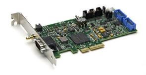
worth of data over the link, almost twice the real world data rate of the USB3 Vision standard and significantly quicker than the latest GigE Vision data rates. This means you can get 2 MP images at 300 FPS! The Aon CXP has been designed for this low cost/high-performance market.
