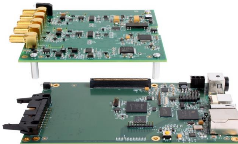
Figure 4. The DT7837 is designed for embedded applications. The I/O block (top board) contains the analog I/O circuitry and the ARM block (bottom board) houses the ARM processor, digital I/O circuitry, and the connectors for communicating with the host computer and other devices.
