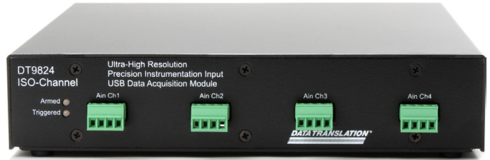
Figure 1. The DT9824 provides ultra-high accuracy and stability while also providing ISO-Channel protection from any noise conditions. Each analog input is galvanically isolated from any other input and has its own return path. This means that other "grounds" or return paths from other signals or from the computer have no possibility to interfere with an ISO-Channel input or return. The shielded steel enclosure, 1U by 1/2 rack, further enhances noise immunity.
