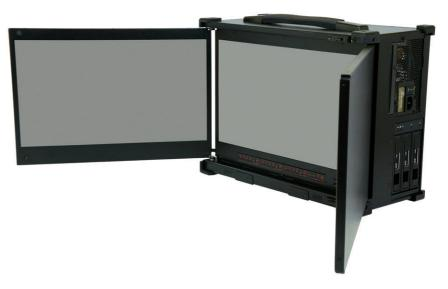
at 5760×1080 resolution. It is capable to fit standard or micro ATX motherboard, one slim optical drive, and three 5.25" devices. Two of the 5.25" bays can be configure into three 3.5" removable HDD or eight 2.5" removable HDD.
