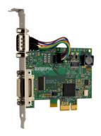
**The PIXCI® EB1-PoCL** frame grabber supports all base configuration Camera Link cameras. When connected to a PoCL camera (Power over Camera Link) with PoCL cable, the PIXCI EB1-PoCL provides camera power.
