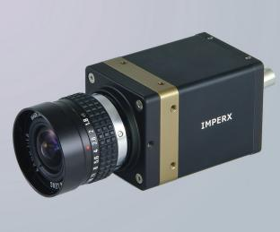
IMPERX ISD-B1921 is an advanced progressive scan, fully programmable CCD camera designed for imaging applications that require high quality images, powerful features and flexibility. The camera is small, light weight, and built around Kodak's KAI-02150 5.5 micron Interline Transfer CCD image sensor with a 2/3" optical format.
