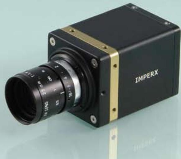
The **IGV-B0610** is an advanced high-speed progressive scan, fully programmable CCD camera designed for imaging applications that require high frame rates, high quality images, and powerful features and flexibility. The camera has a small size, light weight, and is built around Kodak's KAI-0340S Interline transfer CCD image sensor with a 1/3" optical format. IGV-B0610 is available with Ethernet output (GigEVision compliant).
