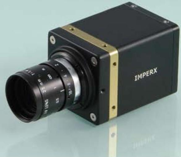
The **IGV-B0620** is an advanced high-speed progressive scan, fully programmable CCD camera designed for imaging applications that require high frame rates, high quality images, and powerful features and flexibility. The camera has a small size, light weight, and is built around Kodak's KAI-0340D Interline transfer CCD image sensor with a 1/3" optical format. IGV-B0620 is available with Ethernet output (GigE Vision compliant).
