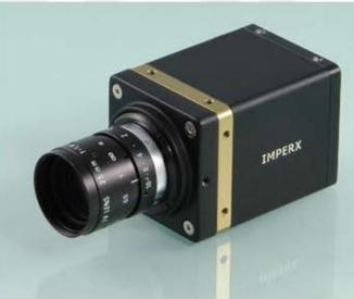
The IGV-B1620 is an advanced high-speed progressive scan, fully programmable CCD camera designed for imaging applications that require high frame rates, high quality images, and powerful features and flexibility. The camera has a small size, light weight, and is built around Kodak's KAI-2020 Interline transfer CCD image sensor with a 1.0" optical format. IGV-B1620 is available with Ethernet output (GigEVision compliant).
